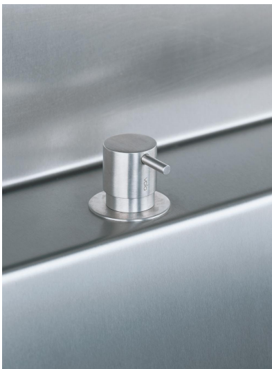
S50 Stop valve with 1/4 turn ceramic disc technology. Includes non-return valve and 1/2" inlet/outlet. Hole cut out size: 30 mm.
