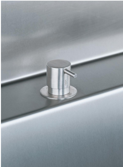
S50 Stop valve with ¼ turn ceramic disc technology. Includes non-return valve and ½" inlet/outlet. Hole cut out size: 30 mm.
